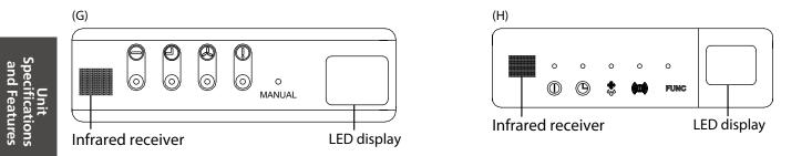
• MANUAL button : This button selects the mode in the following order: AUTO, FORCED COOL, OFF. FORCED COOL mode : In FORCED COOL mode, the Operation light flashes. The system will then turn to AUTO after it has cooled with a high wind speed for 30 minutes. The remote control will be disabled during this operation.
