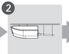
Install the drainpipe
